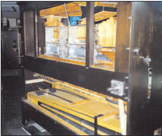
Figure 48. The duplex 165 roll frame arrangement installed in the Nieberle organ by Wurlitzer in 1922 was completely rebuilt by Mike Kitner in the 1990s. Author's photo.
